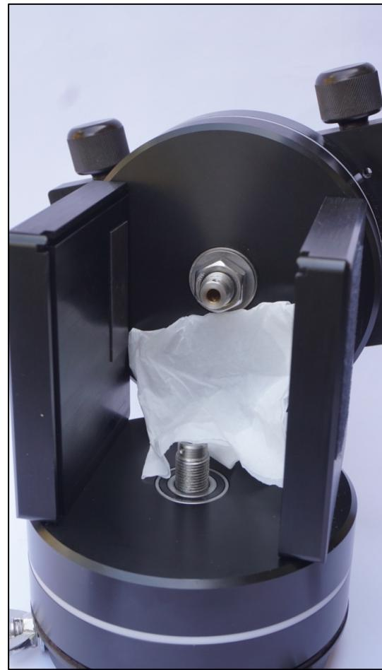
Now remove the protective film from the bottom of the reader to expose the adhesive layer and push the alignment tool with the encoder reader in place in the orientation shown (the encoder jack must point toward the other disk to allow adjusting the friction). Then push the encoder reader down firmly.
