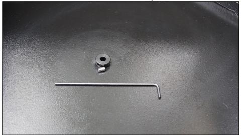
Put the set screw into the threaded hole and make a couple of turns but leave the Allen key in the set screw:
